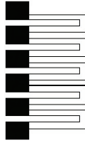
Figure 5. Typical layout of a resistor. The black rectangles represent Al measurement contact pads.
